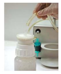
3. Grasp the sides of the filter and pull from the top of the cap. Be careful not to splash any contents that may be in the filter.
