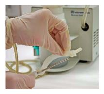
2. Place the nozzle into the affected area and move the nozzle through the spilled mercury.
