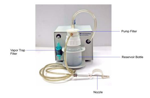
The Mercury QuikVac is simply designed and easy to maintain and operate. It contains a small nozzle, which is used to pick up minor mercury spills. A filter is located between the pump and reservoir bottle to protect the pump from liquid mercury. A vapor trap is also provided downstream of the pump to prevent the escape of mercury vapor.
