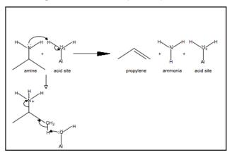
Figure 1. The amine reacts with acid sites to decompose into propylene and ammonia via a mechanism analogous to Hofmann Elimination.
